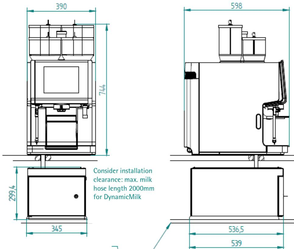
Consider installation clearance: max. milk hose length 2000mm for DynamicMilk
